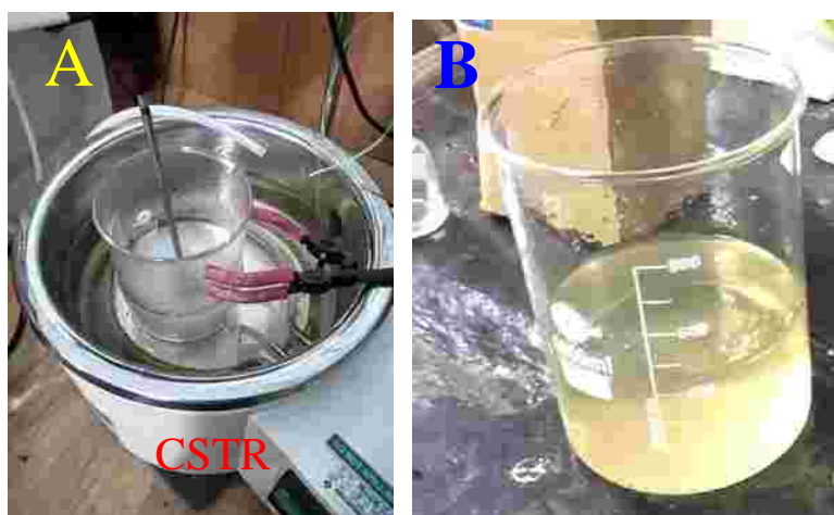
Figure 20. The scheme demonstrate flow reactor set up used for the synthesis of chitosan medication using BPDGE
