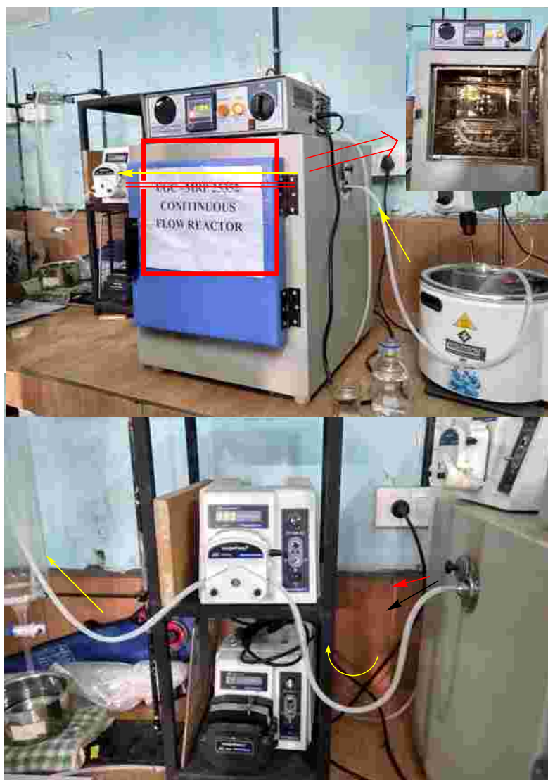
Figure 19. The Flow reactor set up for the Chitosan modification using BPDGE.
