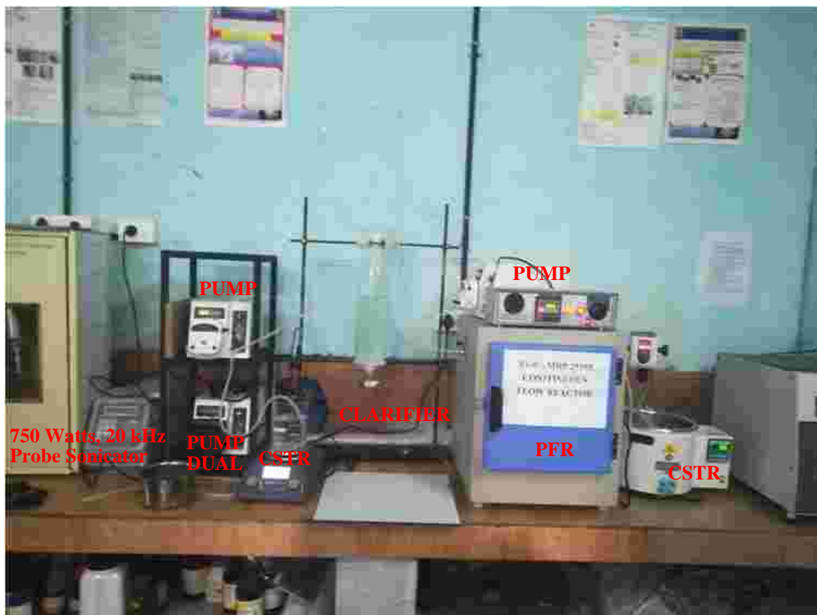
Figure17. The flow reactor set up for the synthesis of chitosan methacrylate/siloxane graft.
